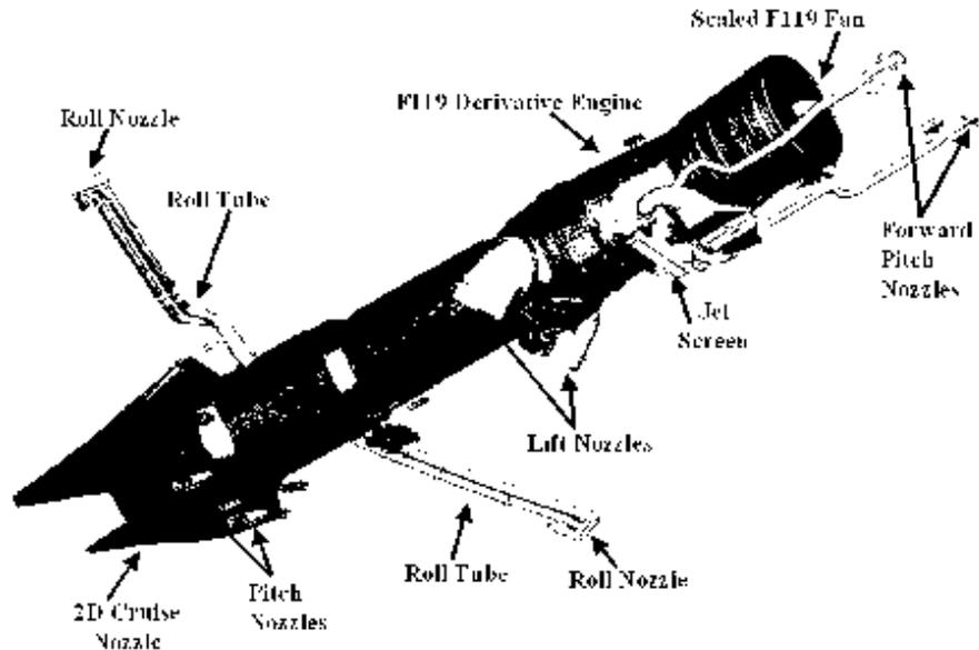
Figure 5.: STOVL propulsion system of X-32B
