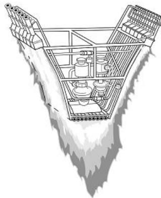
Figure 6. XRS-2200 linear aerospike rocket engine
