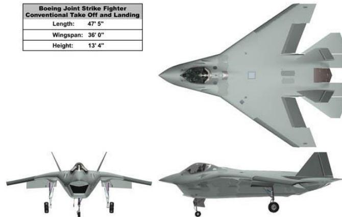
Figure 3. The Boeing Joint Strike Fighter
