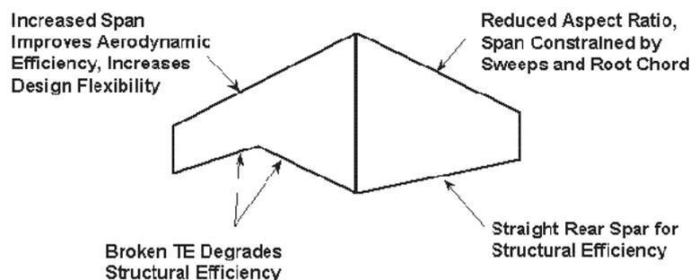
Figure 10. Lambda Wing Advanced Wing Planforms
